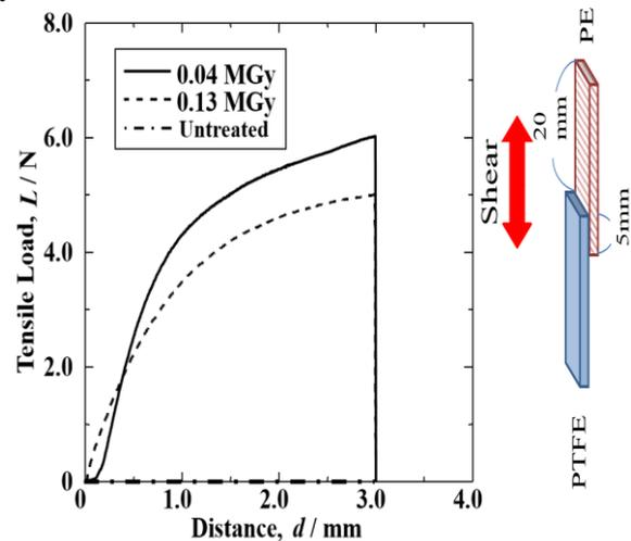
**Figure 2:** Schematic drawing of shearing test and tensile shear stress ( $\tau$ ) strain ( $\epsilon$ ) curves at  $P_s$  of PTFE and PE laminated sheet with and without HLEBI at 0.13 and 0.04 MGy at mean  $P_s$  of 0.50.
