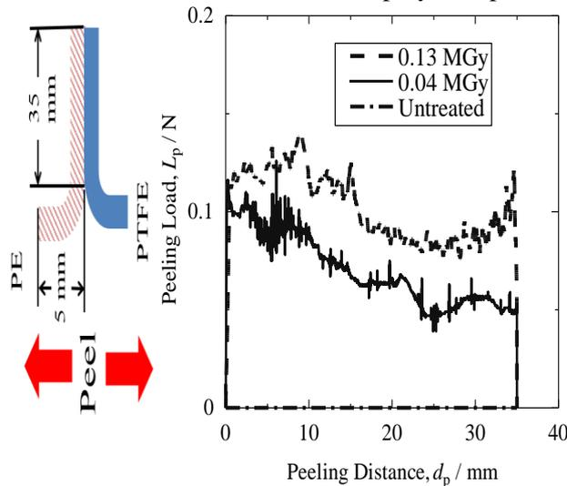
**Figure 1:** Schematic drawing of T-peeling test and adhesive force of peeling resistivity ( $F_p$ ) distance ( $d_p$ ) curves of PTFE and PE laminated sheet with and without HLEBI at 0.13 and 0.04 MGy at mean  $P_p$  of 0.50.
